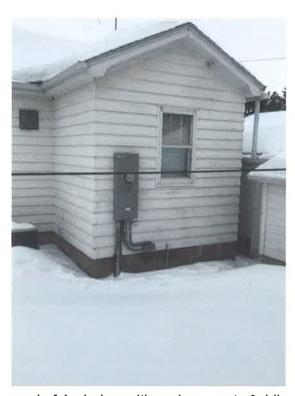
South view. Replacement of 2 windows and removal of 1 window with replacement of siding and siding cover up of removed window.
